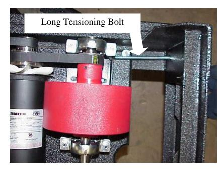
Use a ½" socket wrench to tighten the tensioning bolt just enough to remove the belt slipping. Check the tension on the belt that runs from the motor to the flywheel by twisting or wiggling it. You should be able to twist the belt at least 90 degrees.
