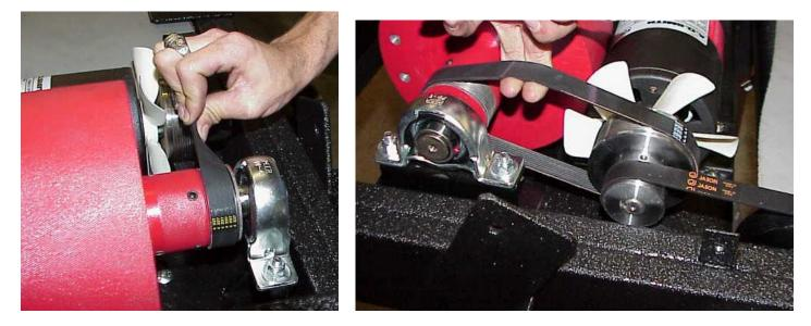
If you wiggle the belt up and down, there should be at least 1" of play. Be careful not to over-tighten the flywheel belt. **Over-tightening the flywheel belt can cause the motor shaft to snap and void the warranty.**
